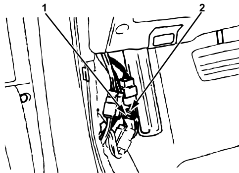
Figure 15-50 1993-94 Legacy ABS Check connector location
