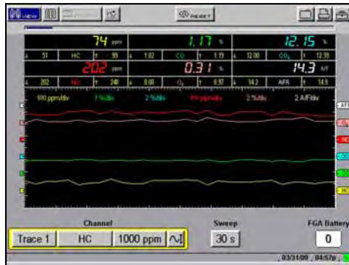
Figure 4-3 Sample Gases test screen
