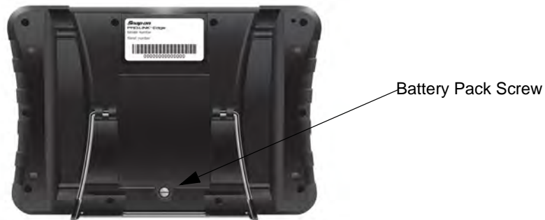
Figure 2.5 Battery Pack Location
