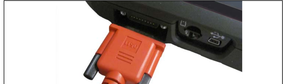
Figure 4-1 DA-4 data cable (26-pin end) connection to diagnostic tool
