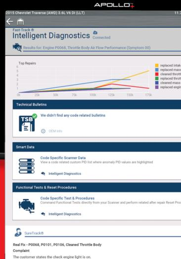
Connected a scan tool and found codes: P0068 - MAP/MAF - Throttle Position Correlation; P0101 - Mas or Volume Air Flow 'A' Circuit Range/Performance and P0106 - Manifold Absolute Pressure/Barometric Pressure Circuit Range/Performance. Inspected the air intake system but found no obvious faults. Using
