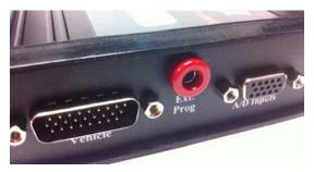
The red *Ext. Prog* banana jack found on the back of the PassThru PRO II takes the place of the "Auxiliary Pin" on the hook up guide below.
