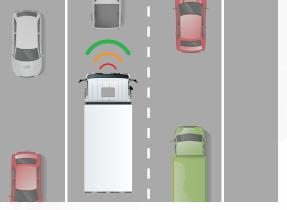
It can be difficult to stay alert during long drives on motorways; Adaptive Cruise Control helps you stay safe. You set your cruising speed and minimum distance from the vehicle ahead. If the vehicle in front slows down, the system reacts and autonomously reduces your speed to maintain the safety distance until the other vehicle moves away or speeds up.
